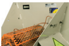
External lubricators to facilitate maintenance
